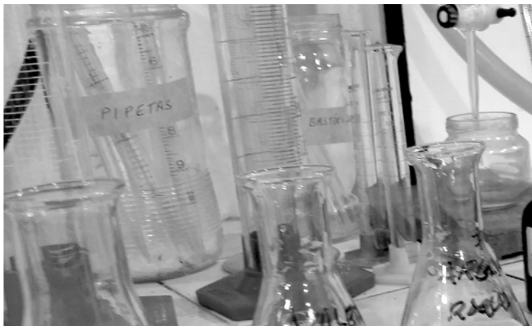
Fig. 5: Assay in the laboratory: qualitative test of soluble salts.
