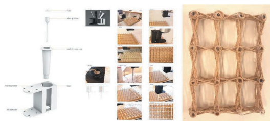
Figure 2. (Left to right) The wicker end-effector tool consists of several parts that can be assembled to perform as a single component for winding, tension control, and precise navigation along specified paths; Fabrication setup and workflow for the robotic winding process; prototype (18 x 12 cm). Authors, 2024.
