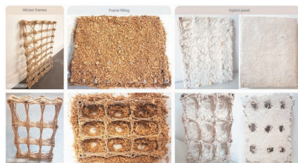
Figure 3. Mycelium – wicker frame compatibility test. Authors, 2024.
