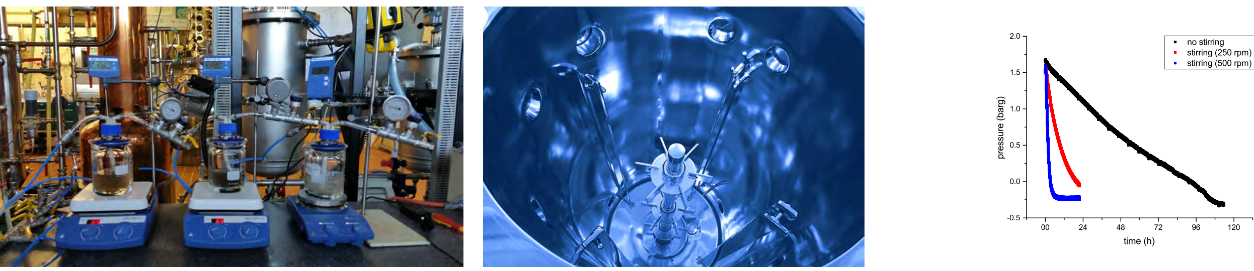
Fig. 3: Left: Methanation in lab scale (0.5l bottles on hot plate magnetic stirrer) with pressure indication. Middle: Pilot plant scale reactor with magnetic stirrer and baffles. Right: Relative pressure in lab scale bottles with and without stirring during biological methanation at 65 °C with Methanothermobacter marburgensis .
