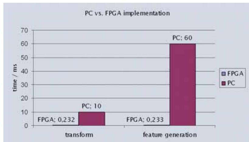
Algorithmenbenchmarking FPGA versus PC
