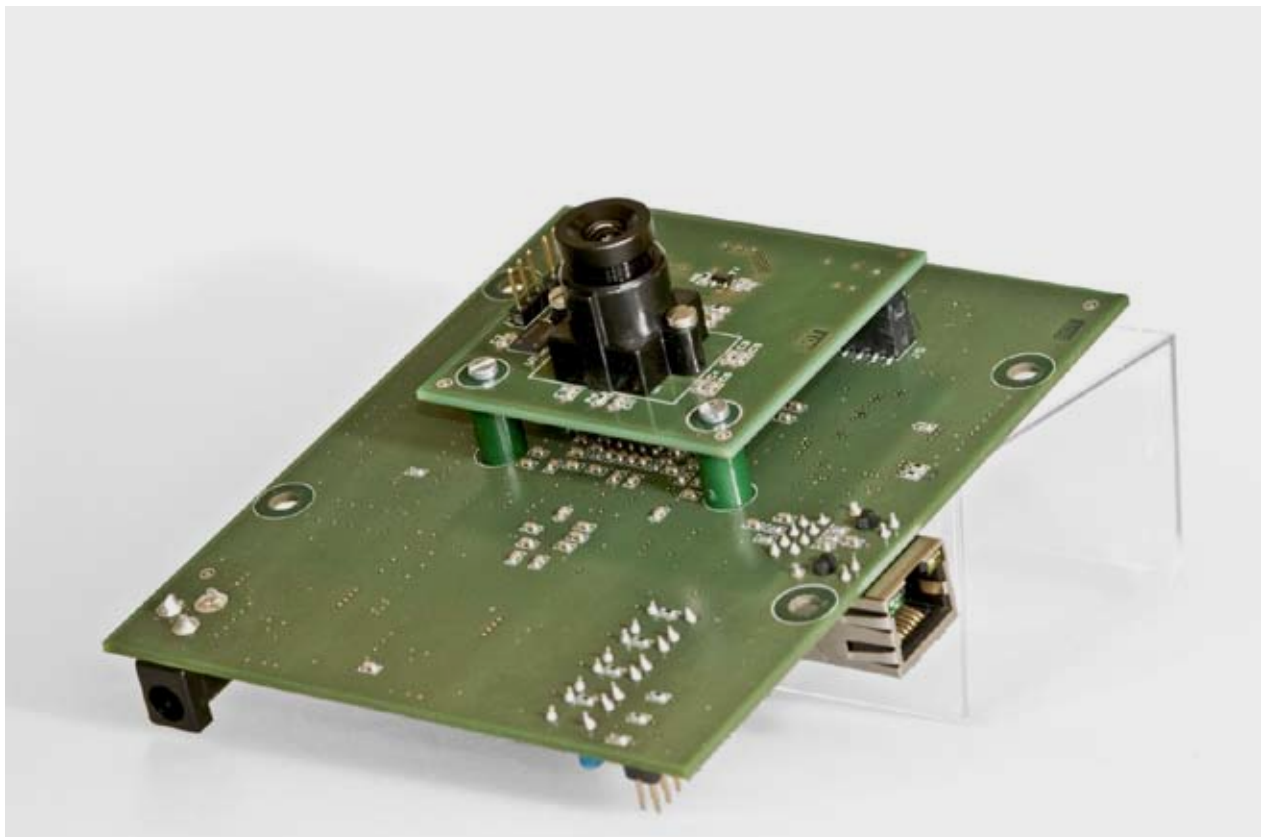
FPGA-Development-Board mit Kameramodul FPGA-Development-Board with camera module
