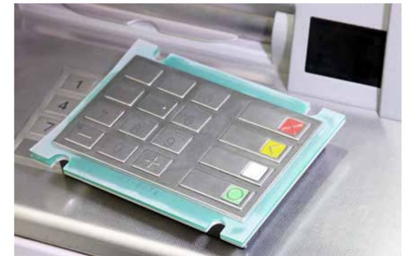
EPP - Encrypting PIN Pad
