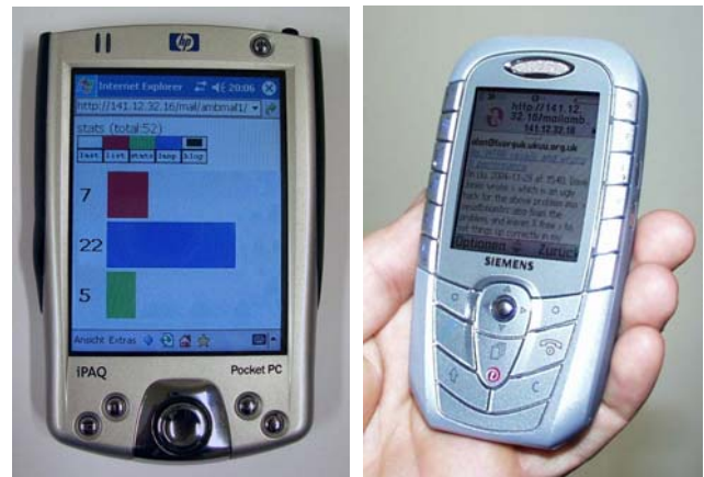
Figure 2: Notification via personal mobile devices: a PDA showing a graphical overview of the inbox (left) and peripheral pop-up notification via a smart phone (right).
