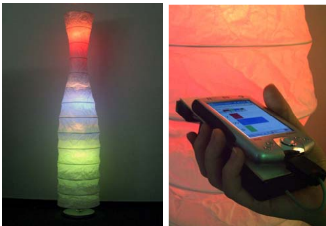
Figure 1: AmbiLamp artefact (left) and direct email access using a PDA with a sensing module (right).
