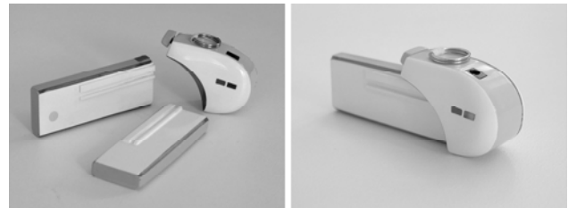
Fig. 5. Personal Aura: The reader module and two ID sticks (left), active Personal Aura (right).
