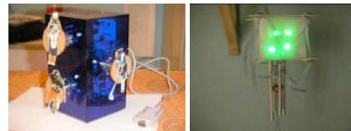
Figure 4 Spinner and Chime: Physical artefacts used to display the status information of instant messenger programs
