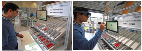
Fig. 3. System setup with projection-based display (left) and HoloLens (right).
