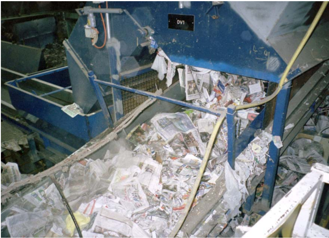
Figure 29 Removing ONP from the belt by blowing air from the bottom in the stream...
