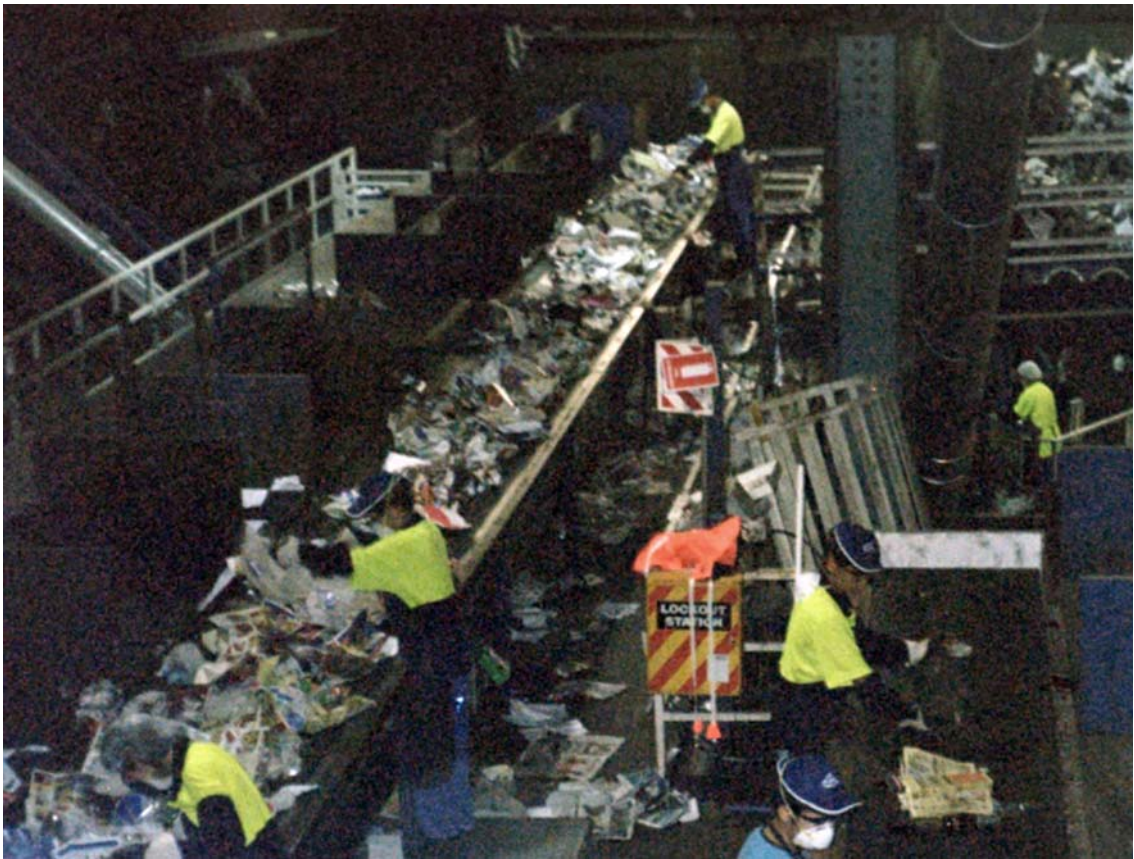
Figure 26 Manual sorting process at Chullora
