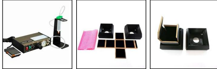
**Fig. 3.** Automatic glue dispenser (*left*), folding aid with a soft cloth (*middle*), folding process (*right*)
