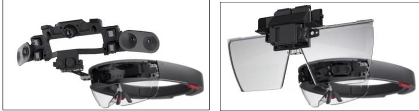
**Fig. 4.** HoloLens: sensor assembly (left) and display assembly (right), images taken from [19].
