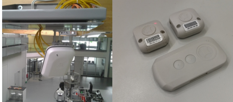
Fig. 3. A sensor of the UWB-system (left) and the associated tags (right).
