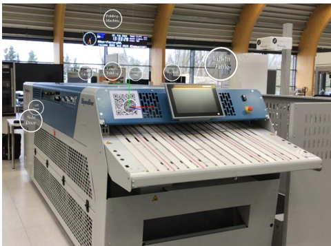
Figure 3: The folding machine located in the SmartFactoryOWL with access points for the explorative mode
