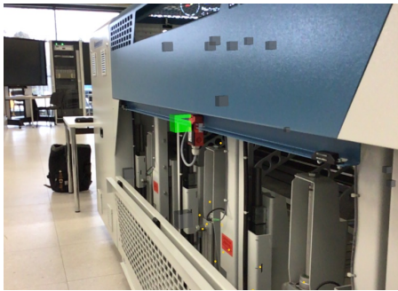
Figure 6: Visualization of active (green) and inactive (gray) sensors
