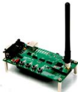
Figure 4: 802.15.4 system with MG2400-F48 transceiver (Radiopulse)
