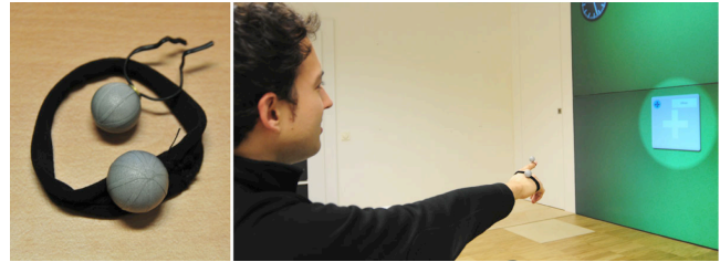
Figure 4. Gesture interface: Tracking is accomplished using reflective markers (left) on the back of the palm and the forefinger (right).
