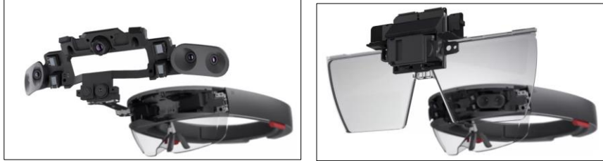
Fig. 4. HoloLens: sensor assembly (left) and display assembly (right), images taken from [19].
