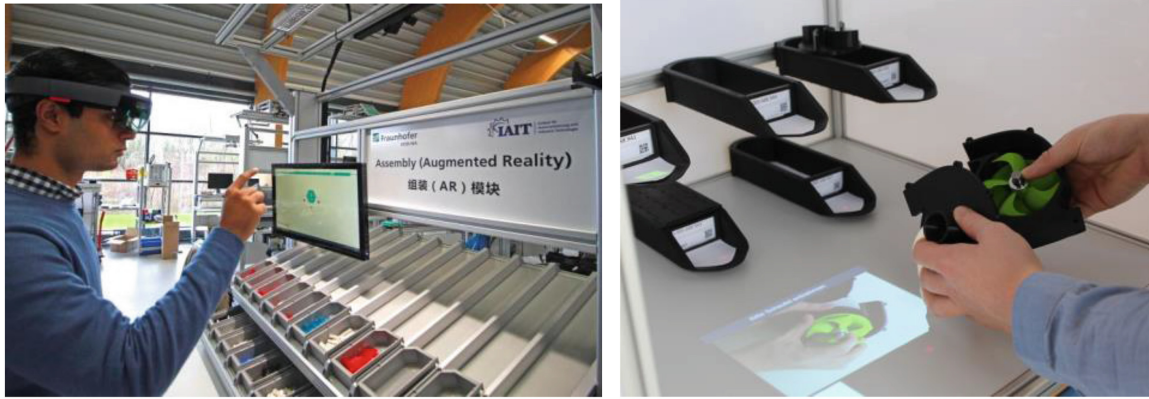
Fig. 3. AR assembly system with AR glasses (left) and projection (right) in SmartFactoryOWL
