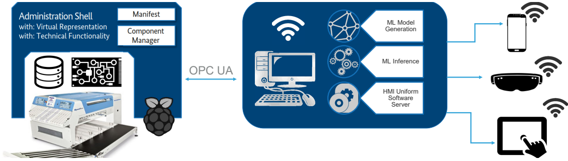
Fig. 2. Structure of the assistance system
