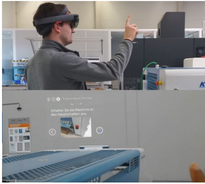
Fig. 3. Human-Machine Interaction, Top: an operator using the assistance system with the HoloLens, Bottom: view of the operator with the HoloLens containing the repair instruction.
